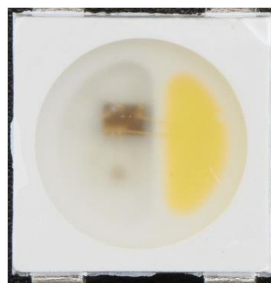
Figure 7: Adafruit neopixel, RGBW-LED, https://www.adafruit.com/product/2758
