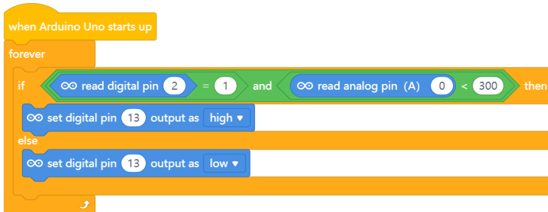
Figure 3: Indicative script for programming the smart light
